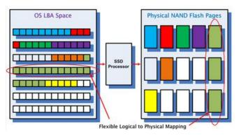
Step 1: "Commands come from the user through the host interface" [2]. The interface can be Serial ATA (SATA) or PCI Express (PCIe). Step 2: "The processor in the SSD controller takes the commands and passes them to the flash controller" [2]. Step 3: "SSDs also have embedded RAM memory, generally for caching purposes and to store mapping information" [2]. Step 4: "The packages of NAND flash memory are organized in gangs, over multiple channels" [2].
